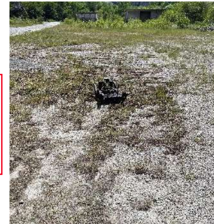
UGV embedded gamma camera and SiPR measurements of lost sealed source
