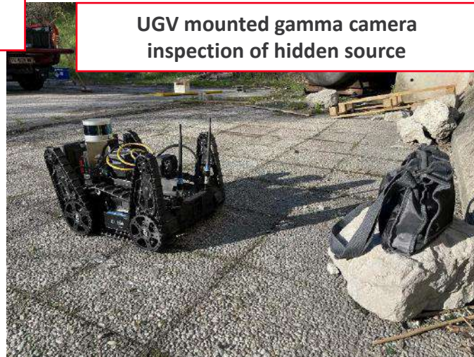
Contamination measurement of abandoned package
