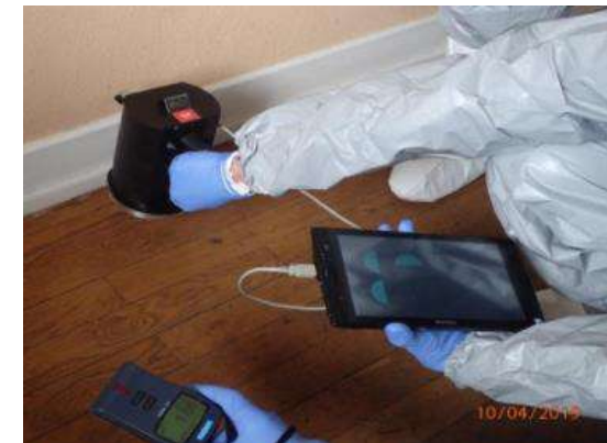
Beta and gamma contamination measurements
