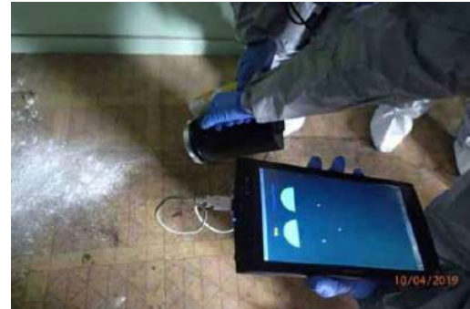
Beta and gamma contamination measurements
