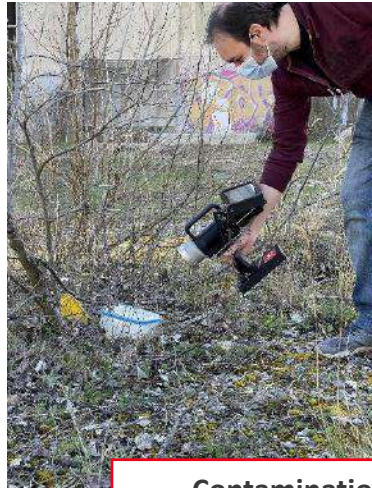
Contamination measurement of abandoned package
